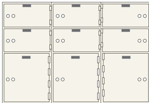
AX-9 (Wt. 195 lbs.) 6 openings ea. 5" x 10" 3 openings ea. 10" x 10"
